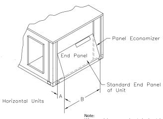
When applying economizer to horizontal units, connecting ductwork must be run full size to allow proper operation of Economizer Damper.
